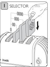
Rotate the 'selector switch' clockwise to the desired number slots you require and insert your frozen slices of bread.
